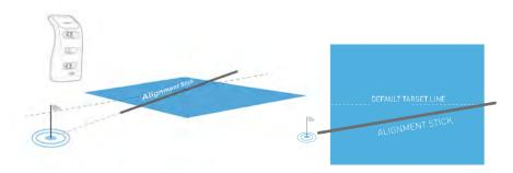
When calibration is complete, the new alignment angle will be shown on the touch display and the LED indicator light will turn solid orange. The new alignment angle will be shown on the touch display.
