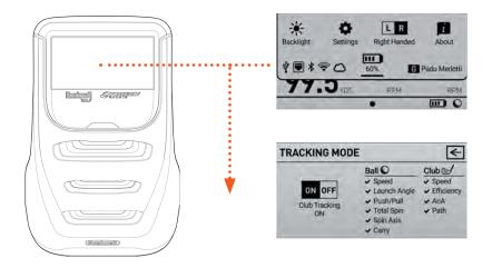
To turn on Club Tracking mode, swipe down to access the QUICK SETTINGS screen, then go to SETTINGS, then TRACKING MODE. Once the ball is in the hitting zone, the Launch Pro will display the READY screen and the green LED indicator light will change from blinking to solid.
