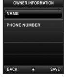
highlight "Phone Number" and press Enter. Scroll to highlight the character and press Enter. To delete characters, scroll to "BKSPC" and press Enter. When finished, press SAVE.
